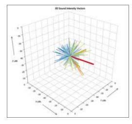
Multidirectional loudspeaker (above) and tetrahedral microphone array (opposite) used for 3D measurements; IRIS plot showing strength, direction and arrival time of a reflected sound (below left); plots measured in the Auckland Town Hall showing variation of reflections at different locations (below right)
